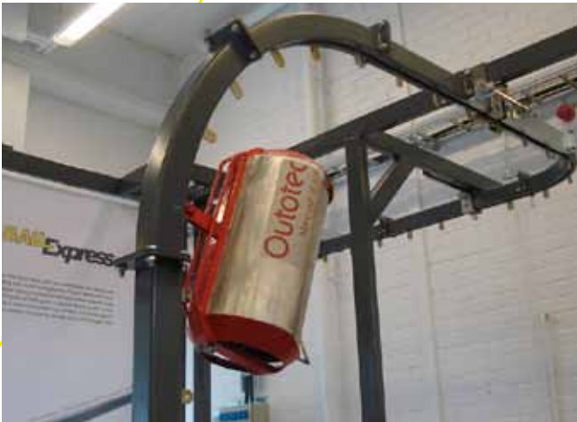
BallExpress, sponsored by Outotec, developed a ball charge system for grinding mills.
